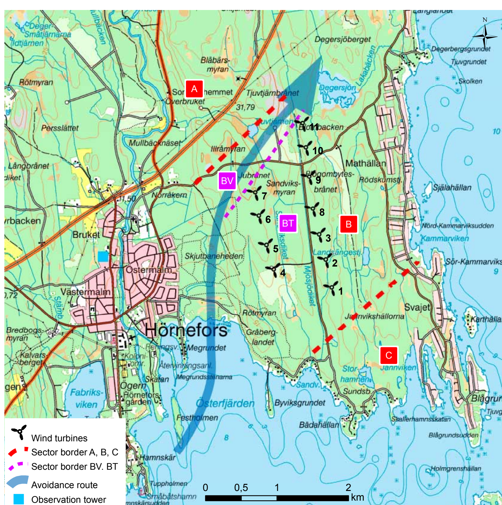
Figure 2. Map over the Hörnefors onshore windfarm showing the location of the wind turbines and the different sectors used when monitoring bird migration routes. Blue arrow shows a common avoidance route for birds flying in sector B.
